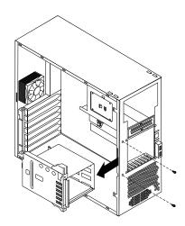
To remove the hard disk drive cage, do the following:
